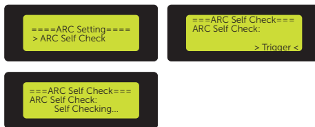
Figure 9-101 Triggering ARC Self Check
