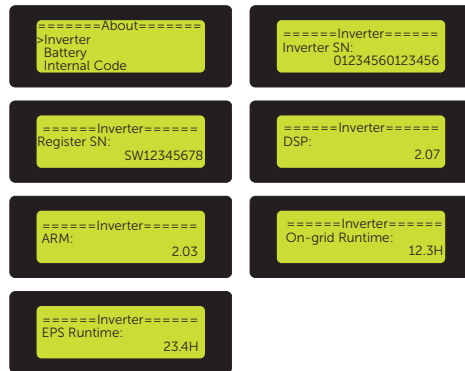
Figure 9-103 Displaying the inverter information
