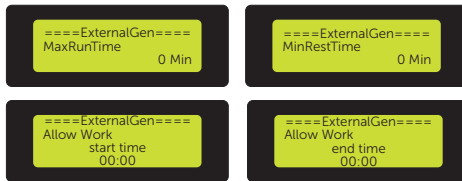
Figure 9-79 Setting MaxRunTime, MinRestTime, allow working period
