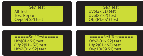
Figure 9-48 Setting to do tests
